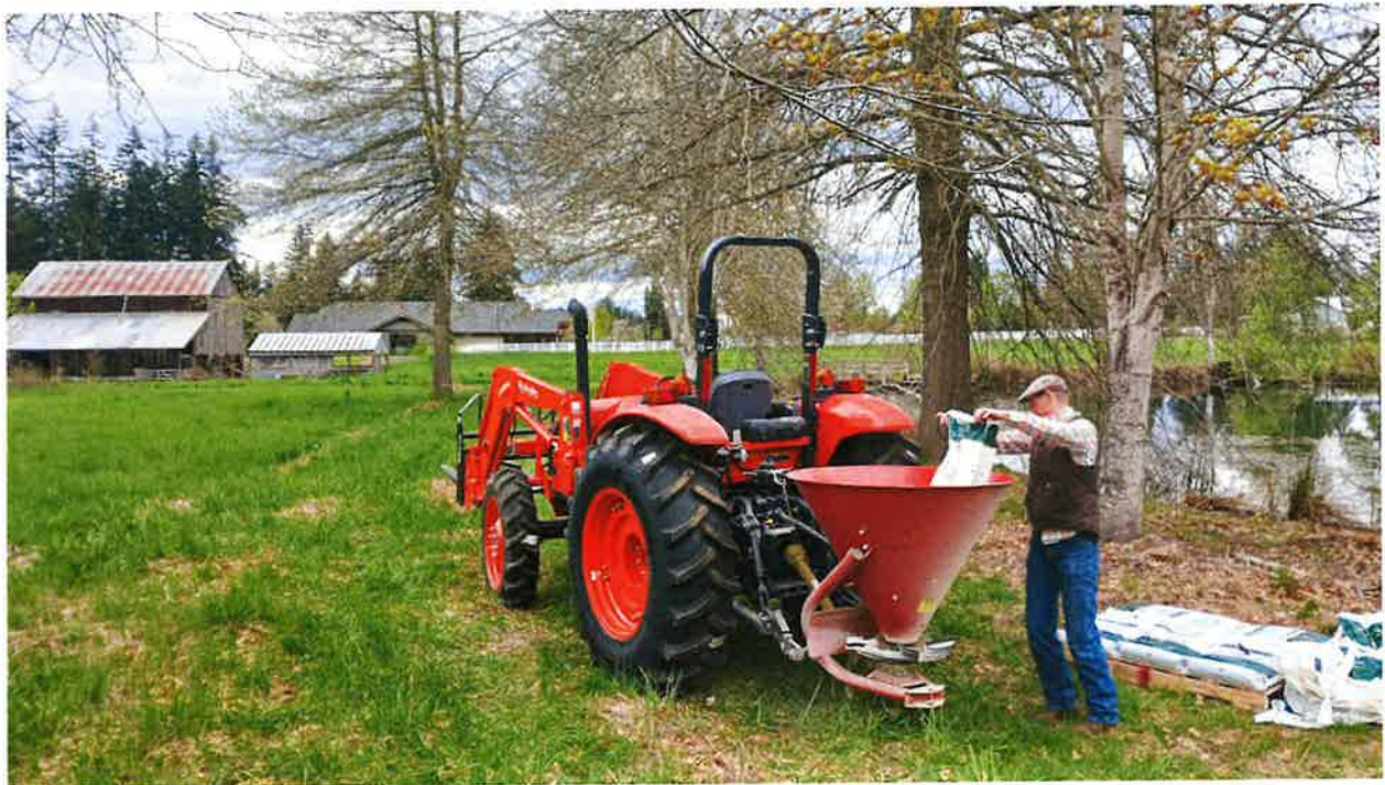
Figure 1 - Gus loading pelletized fertilizer into District's PTO spin spreader for field application
