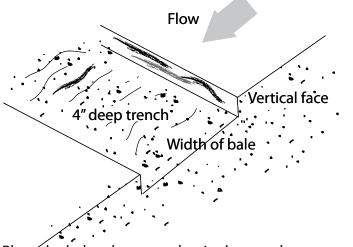
Prepare the trench for the straw bales, perpendicular to the slope. Make the trench 4 inches deep.
